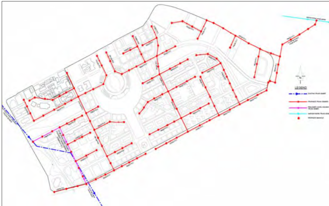
Figure 6-16 Wastewater Collection and Disposal Plan
